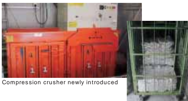
Metal foil reduced to 1/4 of original volume
